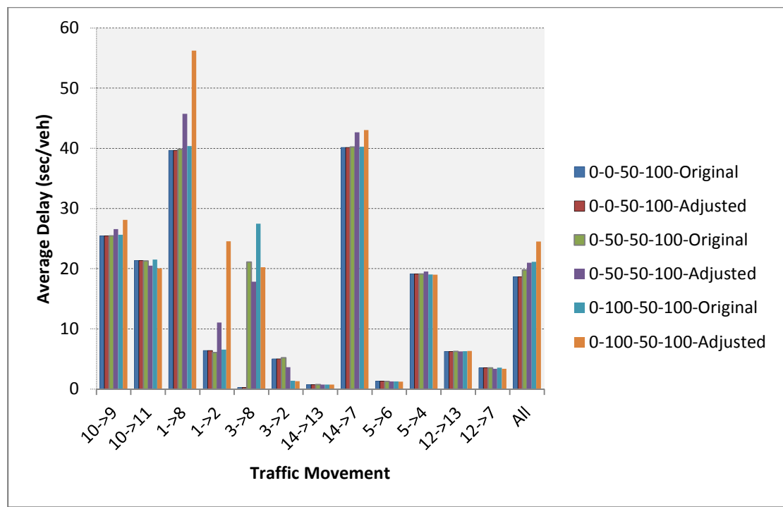
Figure C-36 Average Delay of Fully Actuated Control
