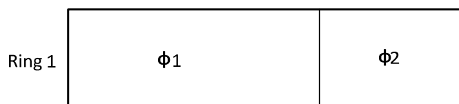
Figure 5-1 Phase and Ring Diagram for the Two-phase Scheme
